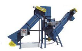
The beverage containers are then discharged onto the out-feed screw conveyor where they run under a fresh water rinse aiding in the removal of residual beverage fluids. The containers are discharged into a waiting container. Incorporate a Model PET Bottle Blower or a baler to make this a complete full beverage container recycling system.
