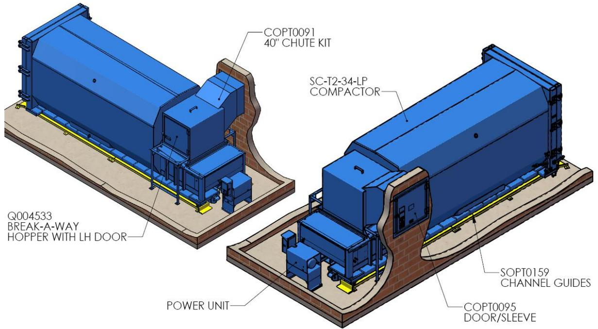
MINIMUM WALL OPENING HEIGHT REQUIRED IS 54.5" FROM COMPACTOR PAD. A 54.5" WALL OPENING WILL PROVIDE 1" OF FALL FROM CHUTE DOOR TO HOPPER. IT IS RECOMMENDED TO HAVE 30° OF SLOPE ON THE CHUTE WHEN POSSIBLE. A 30° WILL ALLOW THE MAJORITY OF MATERIAL TO SLIDE DOWN THE CHUTE WITHOUT IT BUILDING UP ON THE CHUTE SLOPE. TO OBTAIN A 30° SLOPE ON THE CHUTE FOR THE SHOWN LAYOUT THE BOTTOM OF THE WALL OPENING NEEDS TO BE AT 68" ABOVE THE COMPACTOR PAD
