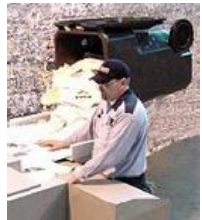
Shown tipping onto the feed table of a Series 1 industrial paper shredder.
