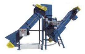
Product is loaded on the in-feed conveyor hopper and is conveyed up into MV PERF mechanism where the containers are perforated and crushed with the beverage fluid discharging into the (optional) capture tank.
