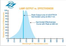
Our 254nm germicidal lamps are used extensively in the <u>air and water purification</u> <u>markets</u> and have been utilized in applications such as food and beverage, medical, HVAC (Heating, Ventilation and Air Conditioning), pharmaceutical, the semiconductor sterilization industries and many others. Our germicidal lamps are essential components in many municipal drinking water facilities, waste water and ground water remediation industries.
