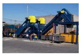
With the optional scale and indicator, the operator can record the weight, trip the weigh hopper door, and discharge the aluminum into the optional HV extreme volume can crusher for volume reduction prior to baling. The entire buy-back process can be handled with only one employee, reducing your labor costs and increasing your profits!
