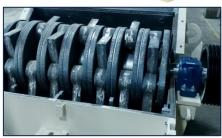
Hammers up to 90 pounds each are two way reversible cast manganese for the longest possible wear life.
