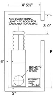
Typical Installation For XM40 / XM40M
