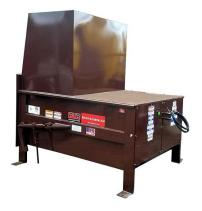
Our TP-3000SP (short profile) compactor was our response to customers battling space constrictions and those who could not accommodate a long chute. We managed to construct a twin cylinder machine with high compaction forces and an overall length of 145 inches.
