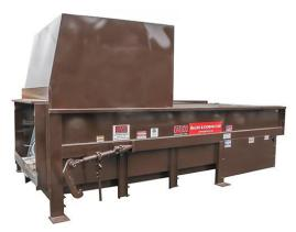
Our TP-3000HD compactor is designed for long lasting performance and durability. All components are built using heavy-duty structural steel components and welded by AWS certified technicians. This unit has total U.L. approval, standard 3 button controls (on/off key switch, mushroom stop, auto reverse) and a 13' Sealtite.
